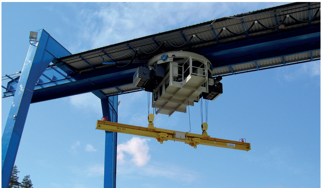
Lifting beam with adjustable lifting points
