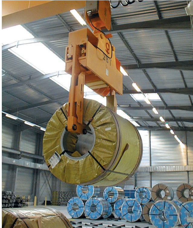
Head-fitting and length of gripping legs manufactured to suit your application
